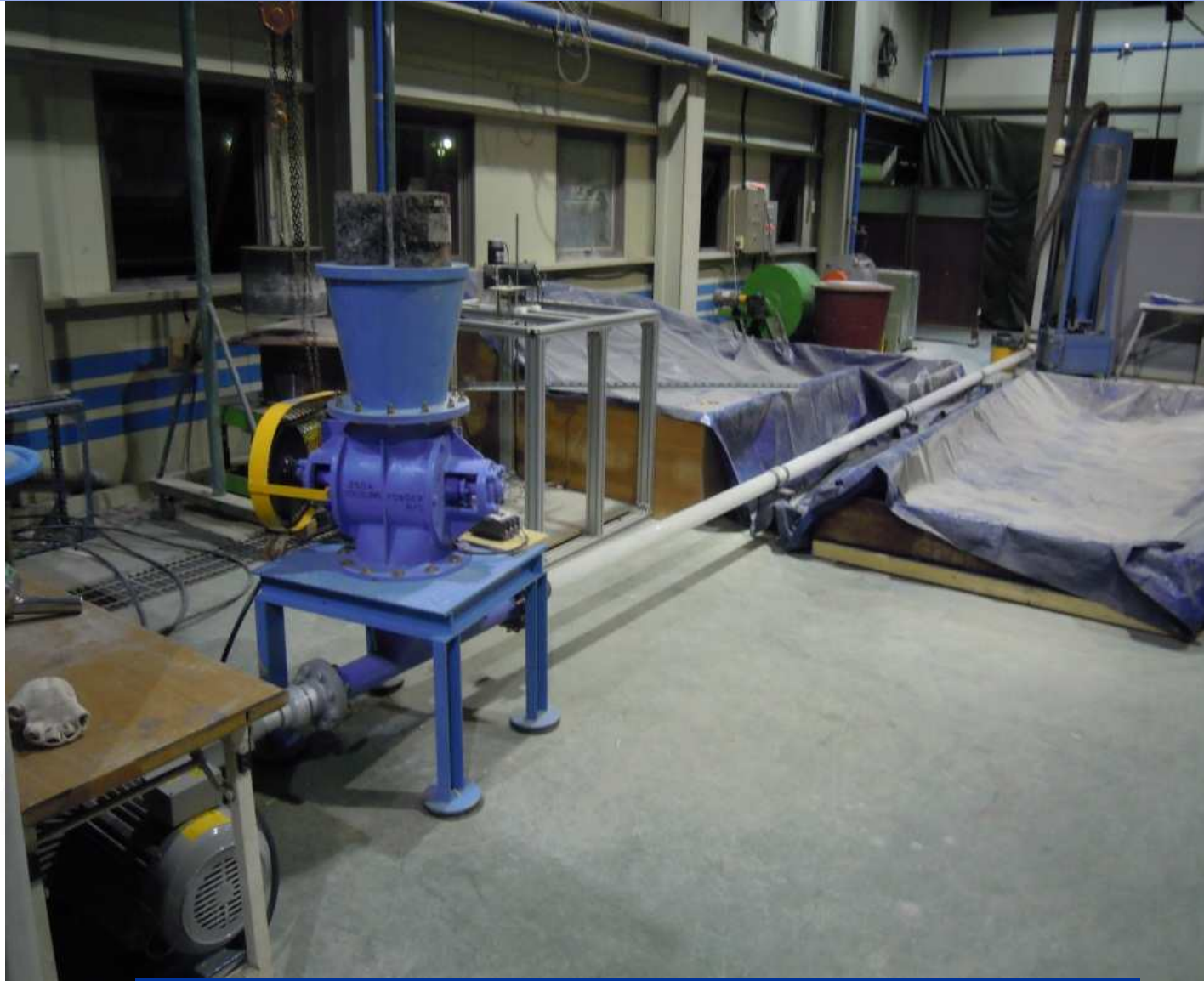
c Pneumatic Transportation System Prototype
