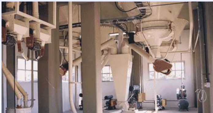
Pneumatic Conveying in the Flour Mill Facility
